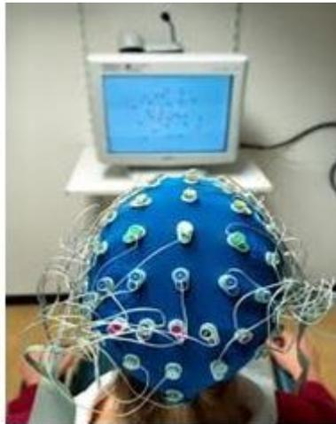
**Figure 2.2: An EEG cap for the use of a large number of electrodes.**
