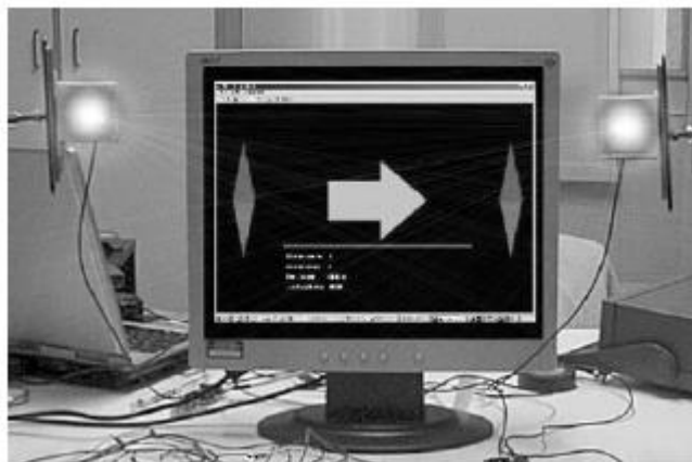
Figure 3.2: A Detail of BCI Simple Setup Screen Center and the Two LEDs Left and Right [14].
